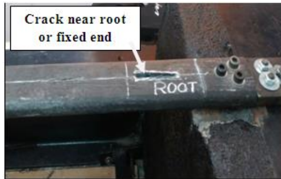
Figure 3: Damaged beam by producing crack near root Figure 4: Damaged beam by producing crack at mid
