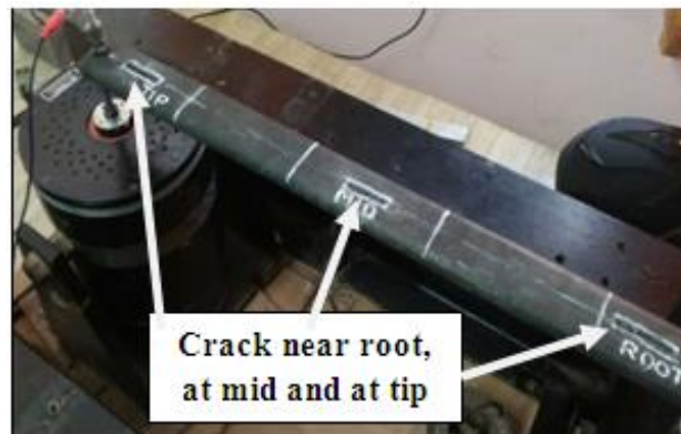
Figure 5: Damaged beam with multiple cracks
