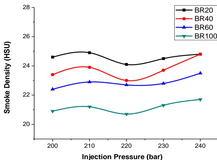
Figure 3: Injection Pressure vs. Smoke Density
