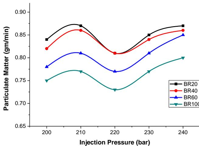
Figure 7: Injection Pressure vs. Particulate Matter
