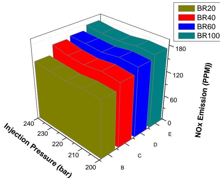
Figure 10: Injection Pressure vs. NOx Emission
