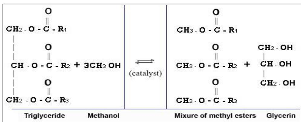
Figure 1: Transesterification Process
