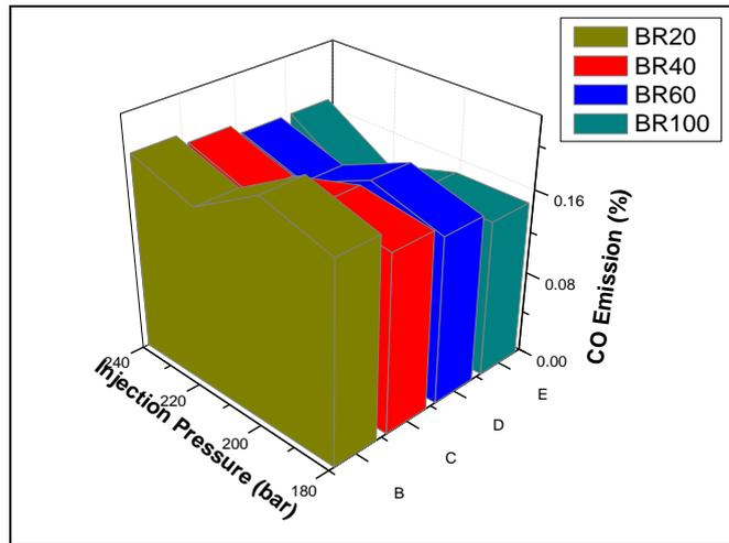
Figure 6: Injection Pressure vs. CO Emission
