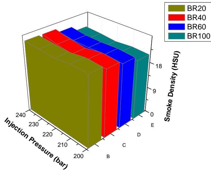
Figure 4: Injection Pressure and Smoke Density
