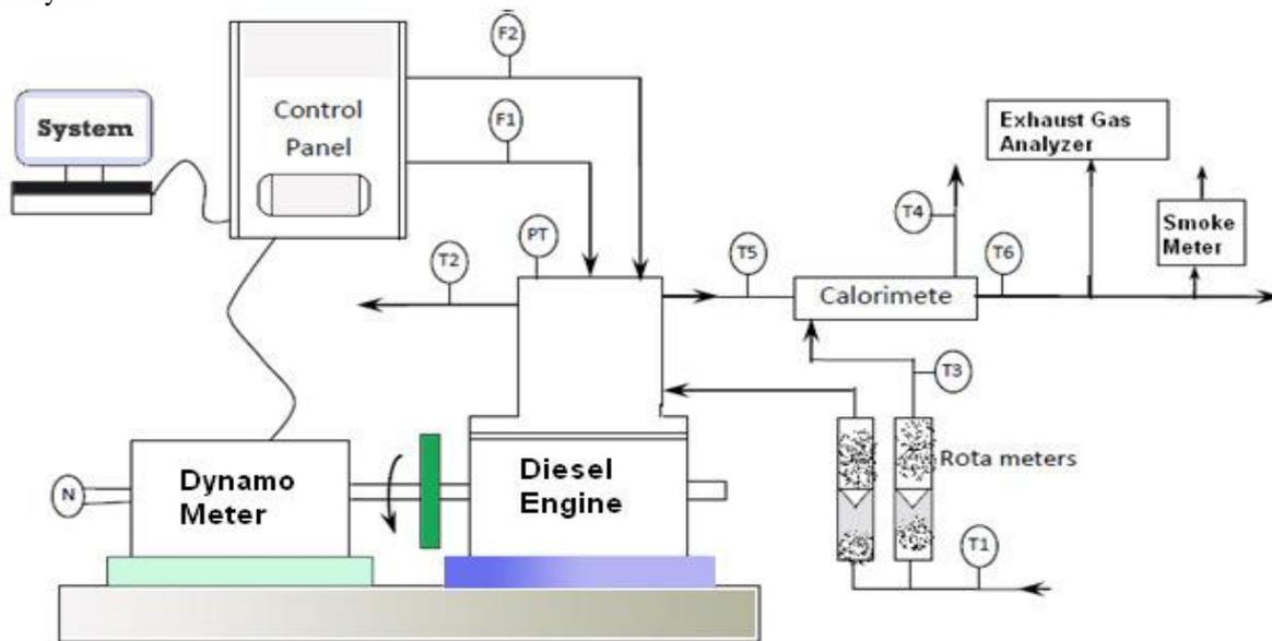
Figure 2: Schematic Diagram of Experimental Setup
