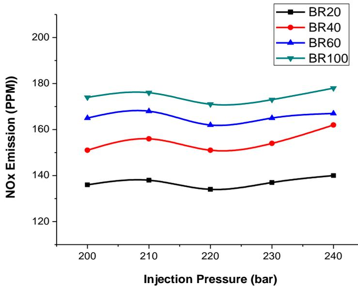
Figure 9: Injection Pressure vs. NOx Emission
