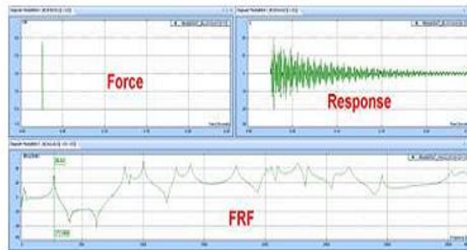
Fig 5- Experimental impact hammer modal testing data
