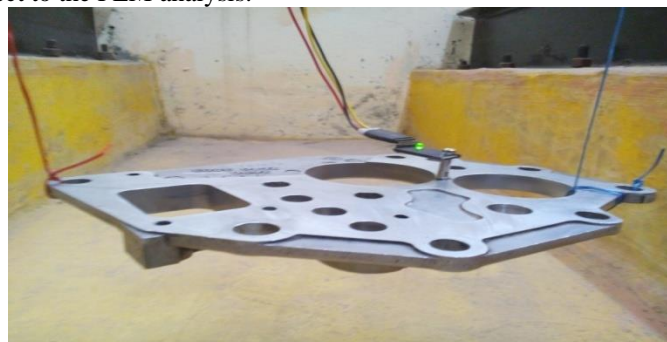
Fig 6 (a)-Photograph of modal testing
