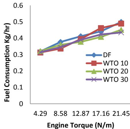
Fig 8: Variation of fuel consumption with engine torque for DF and WTO blends.
