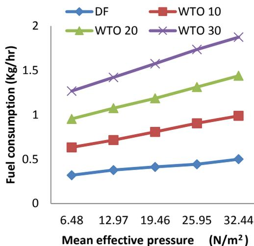
Fig 10: Variation of fuel consumption with mean effective pressure for DF and WTO blends
