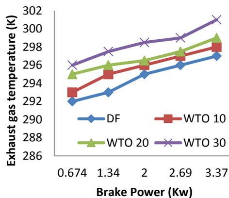
Fig 9: Variation of exhaust gas temperatures with brake power for DF and WTO blends.
