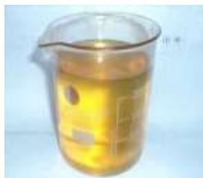
Fig1: pure transformer oil
