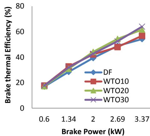
Fig 6: Variation of brake thermal efficiency with brake power for DF and WTO blends.
