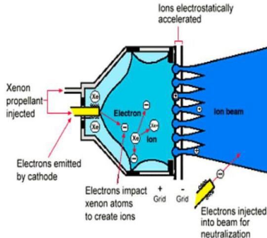
Fig 6: Xenon Ion Engine
