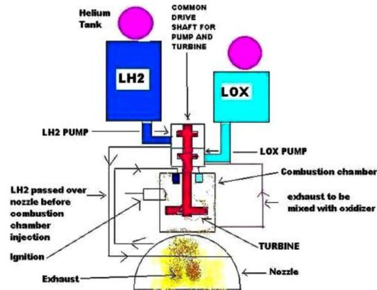
Fig 5: Complicated Staged Combustion Engine for Increasing Efficiency
