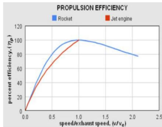
Fig 2: Propulsion Efficiency Curve
