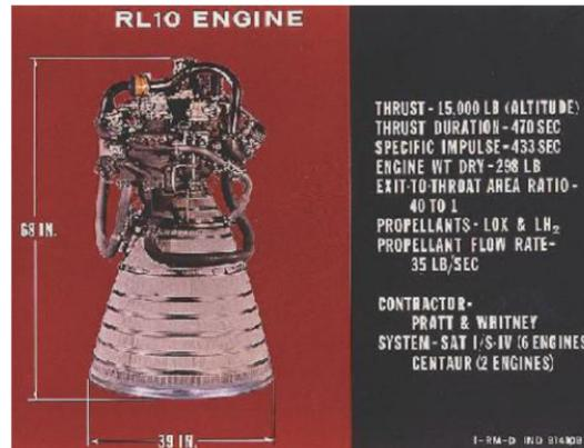
Fig 3: Details of RL-10 Cryogenic Rocket Engine
