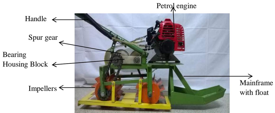
Figure 3.1: Details of Semi Automatic weeder
