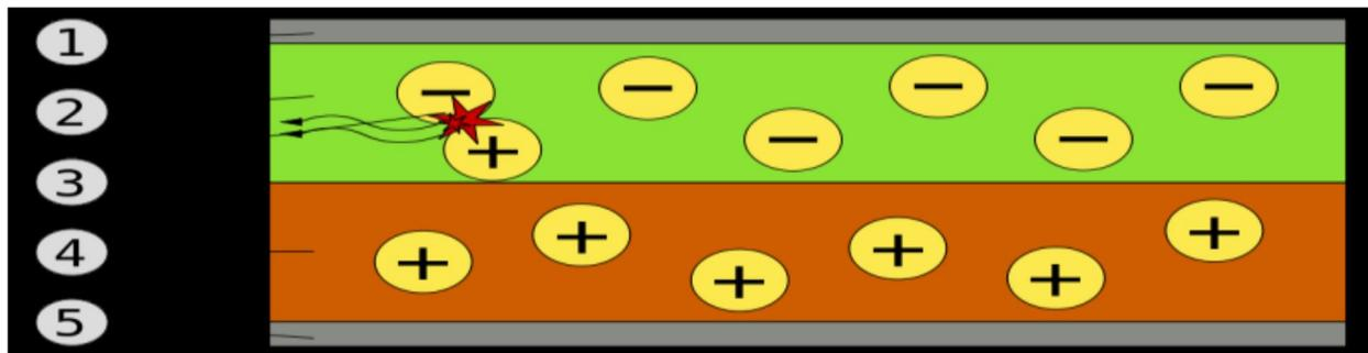
Figure2: Schematic of a bilayer OLED: 1. Cathode (-), 2. Emissive Layer, 3. Emission of radiation, 4. Conductive Layer, 5. Anode (+)
