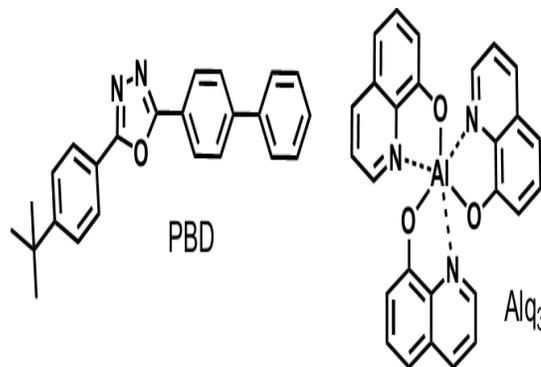
*Figure 1 : Commonly used components in electrons transport layer.*
