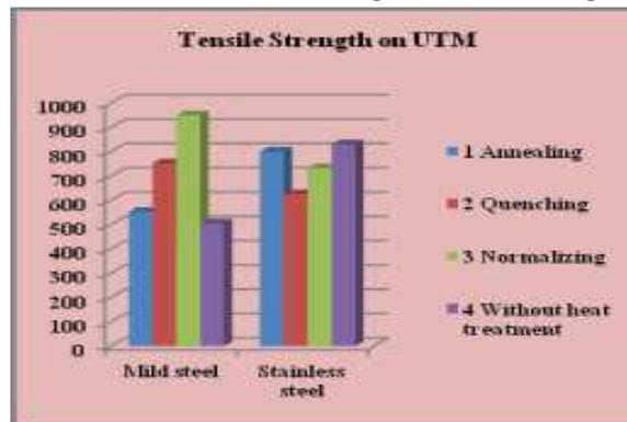
Figure.4 Results of Tensile strength
