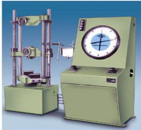
*Figure3. Universal testing machine*
