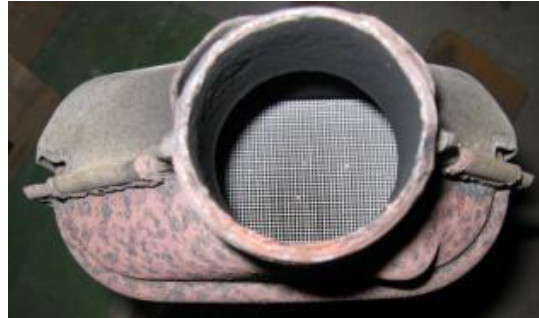
(b) Ceramic -core converter
