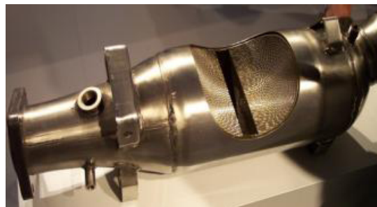
Fig 6.1: (a) Cutaway of a metal-core converter
