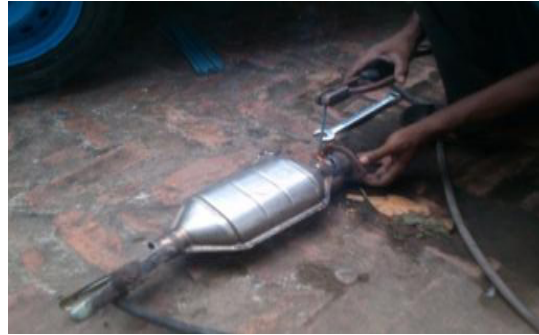
Fig 2: Catalytic converter to be welded in exhaust system of the car, Toyota E-90 in MIST welding shop.
