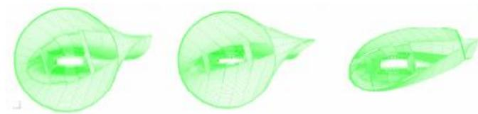
**Figure 7. Meshes obtained with three different aerofoil series.**
