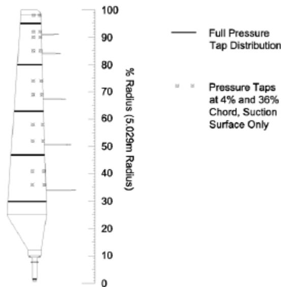
**Figure 11. Blade cross-section and planform, showing pressure tap locations.**
