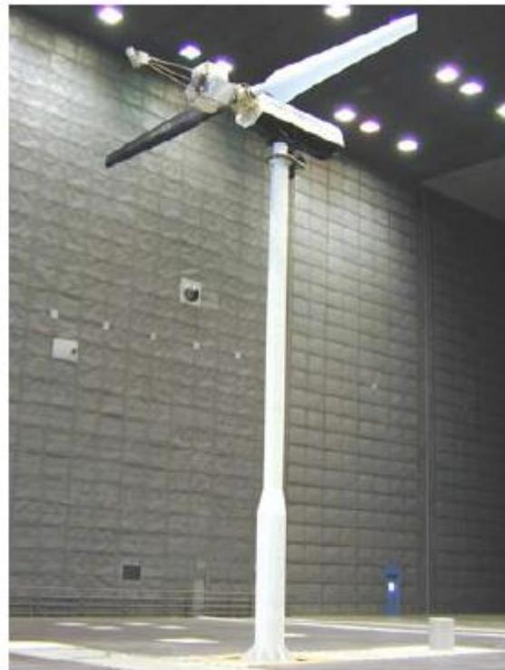
**Figure 10. NREL Unsteady Aerodynamics Experiment wind turbine in NASA Ames 80 ft x 120 ft wind tunnel.**
