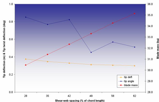
Figure 6. Shear-web placement sweep results.
