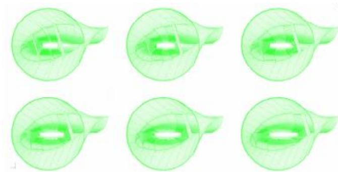
Figure 5. Meshes obtained in shear-web transverse placement analysis.
