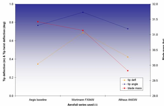
**Figure 8. Aerofoil series sweep results.**
