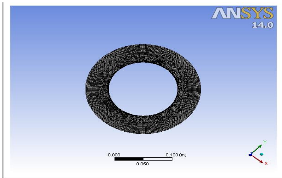
Fig. 2. Meshed model of bore surface
