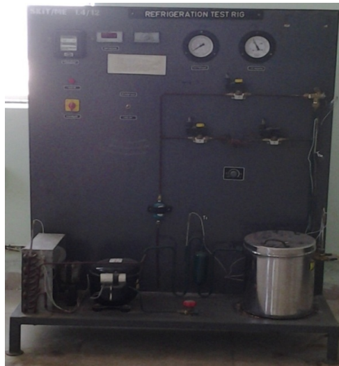
Experimental Set Up (Refrigeration Test Rig)
