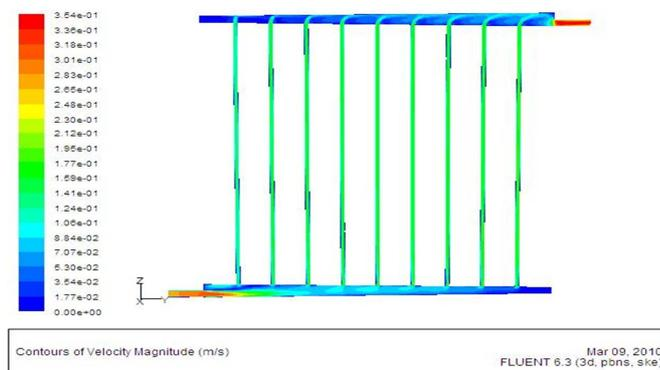
Fig.5 Variable header system
