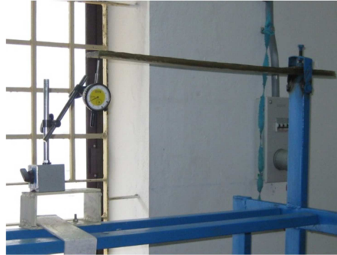
Figure 3: Deflection test arrangement
