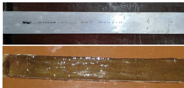
Figure 2: Specimens of Aluminium & GFRP
