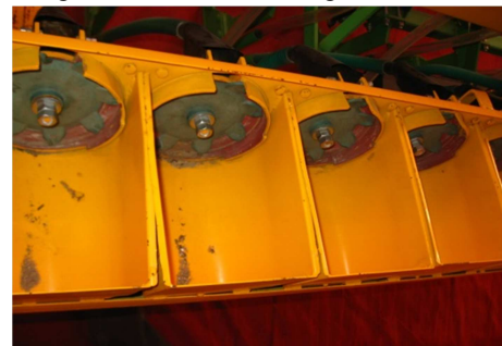
Figure1 (b) Seed metering mechanism
