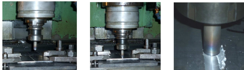
Fig. 2 Stages of friction stir welding experimental Process
