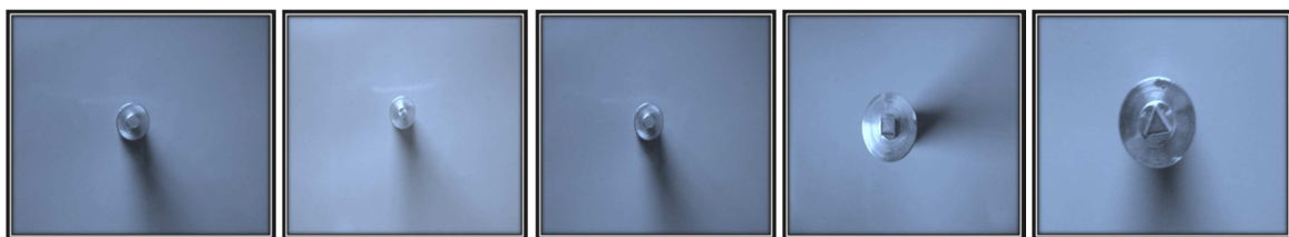
Fig.4. Straight cylindrical, Tapered, Threaded cylindrical, Square and Triangular profiled tools
