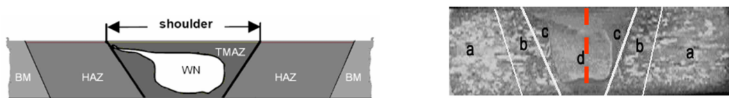
Fig 3 Different zones of FSW joint at the weld.
