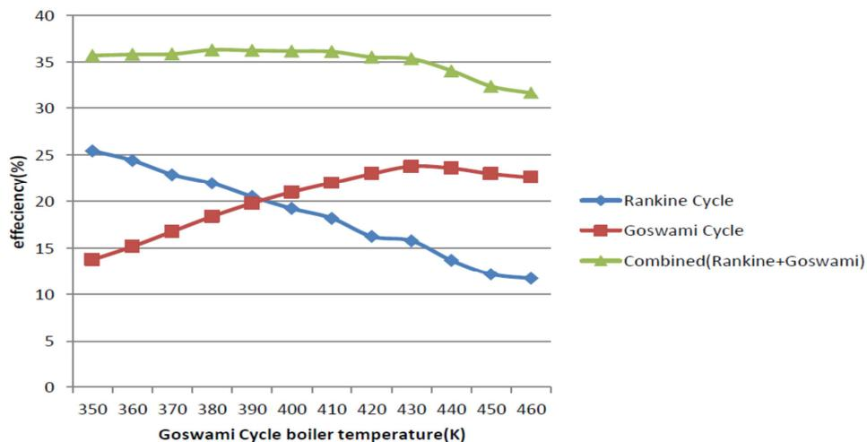
**Figure: 4** Efficiency of Rankine, Goswami and Combined Cycle (Rankine + Goswami) at various Goswami Cycle boiler temperatures.
