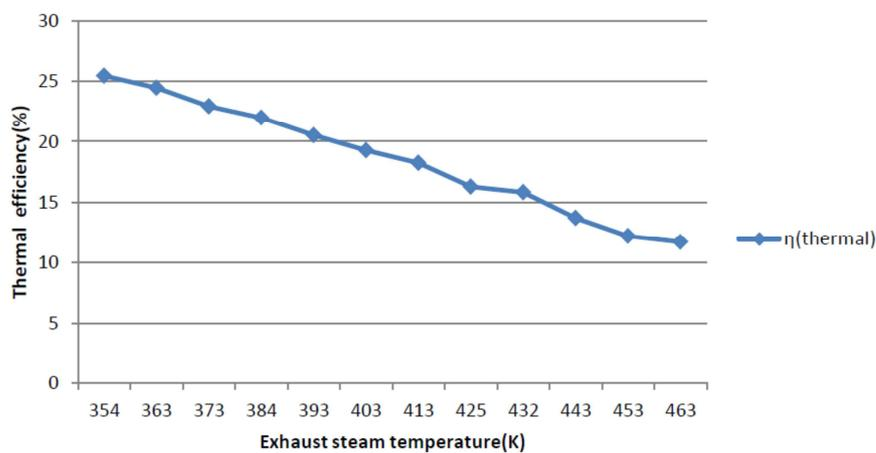
**Figure: 2** Variation of thermal efficiency of Rankine Cycle with exhaust steam temperature
