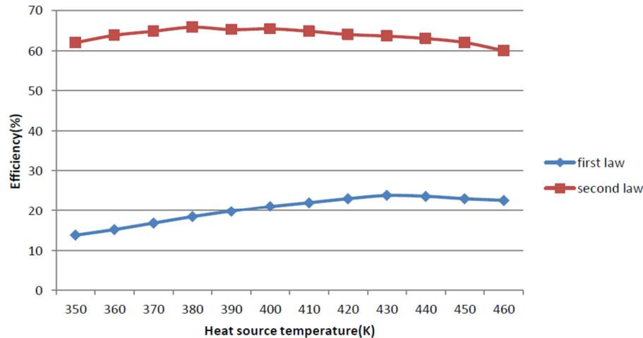
**Figure: 3** Efficiencies of Goswami Cycle at various heat source temperatures
