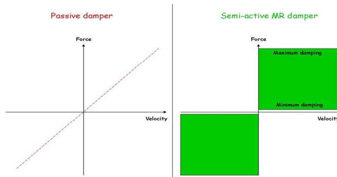
Graph 4.1 – Passive Damper Characteristics vs. Semi-active MR Damper Characteristics
