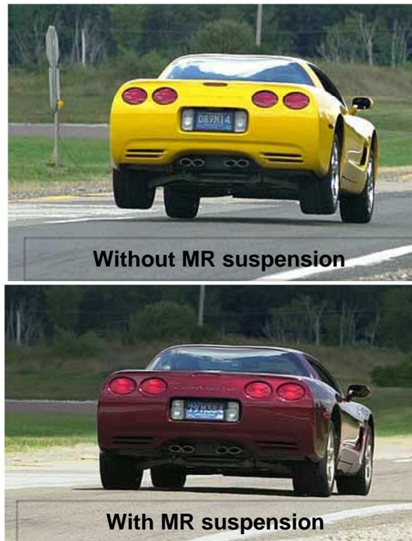
Picture 4.1–Base C5 Corvette and 50th Anniversary Corvette with Magnetic Selective Ride Control Suspension [13]
