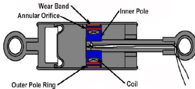
Figure 4.2 – Schematic Drawing of an MR Fluid Damper [5]
