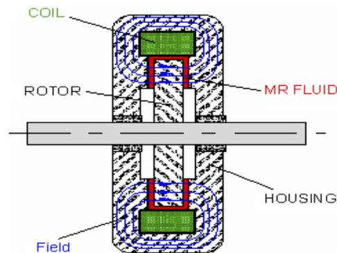
Figure 4.1: MR Fluid Rotary Brake [4]
