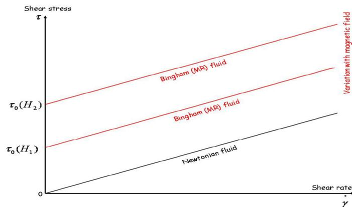
Graph 2.1 – Shear Stress vs. Shear Rate for Newtonian and Bingham (MR) Fluid [4]
