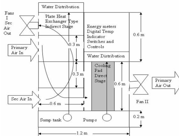
Figure 2. Experimental Set Up IEC/DEC [11]
