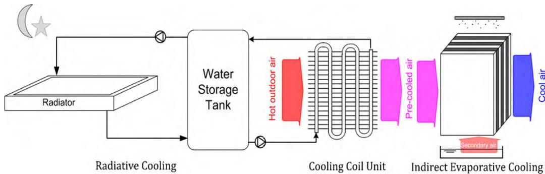
**Figure 3.** System of radiative cooling and cooling coil assisted IEC [17]
