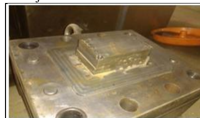
Fig.4.8. Core side assembled view
