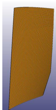
Figure 2: Structure of blade used for simulation
