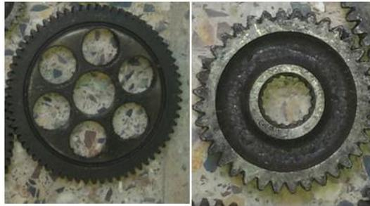
**Figure 2:** Driven Gears, **Figure 3:** Driver Gear
