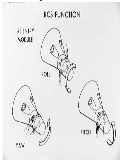
Fig 2 Functions of RCS during Re-Entry
