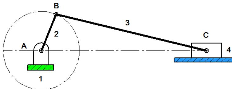
Fig.4 Slider crank mechanism
