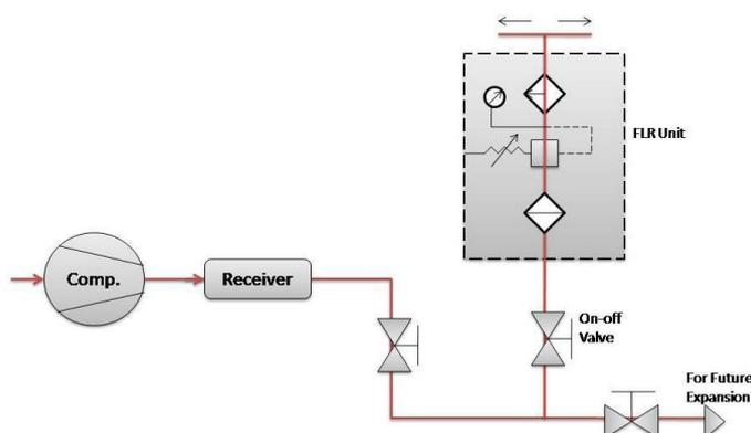
Fig. 1 Basic Pneumatic System
