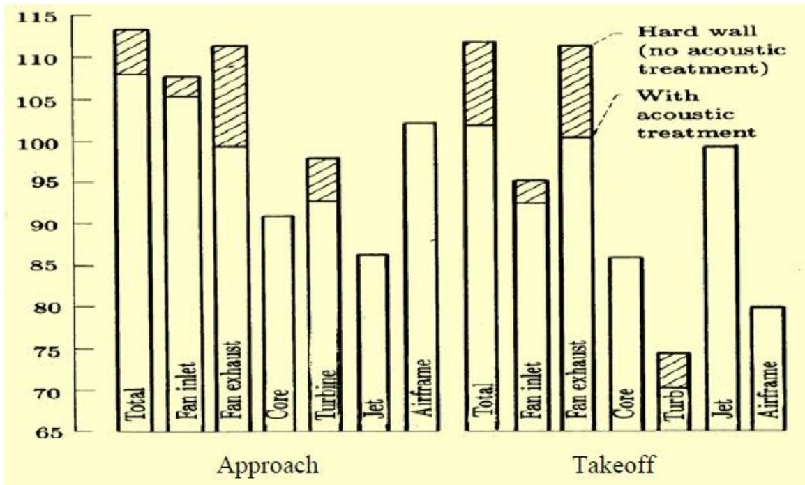
Figure 1. NOISE DISTRIBUTION IN HIGH BYPASS RATIO AIRCRAFT
