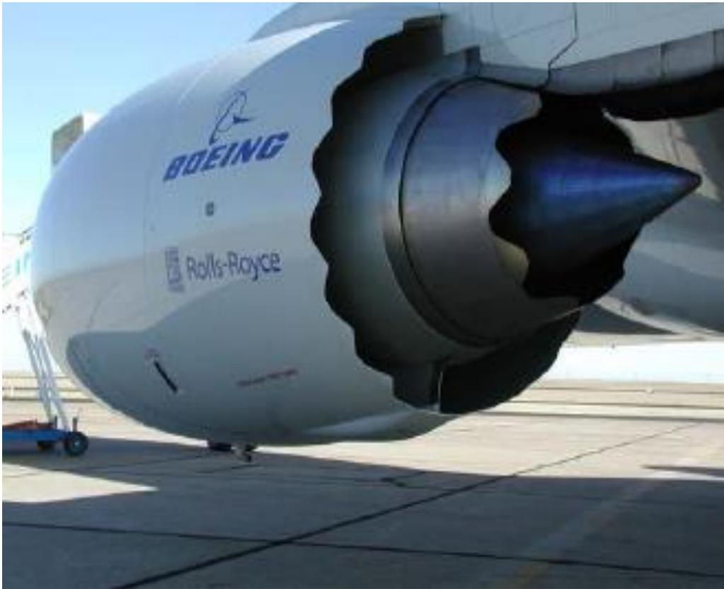
Figure 2. INCLUSION OF CHEVRONS IN COMMERCIAL AERO ENGINE.
