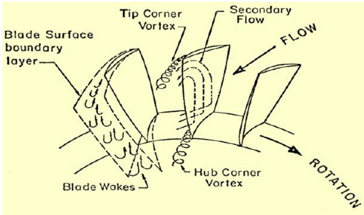
Figure 3. TRAILING EDGE NOISE GENERATORS
