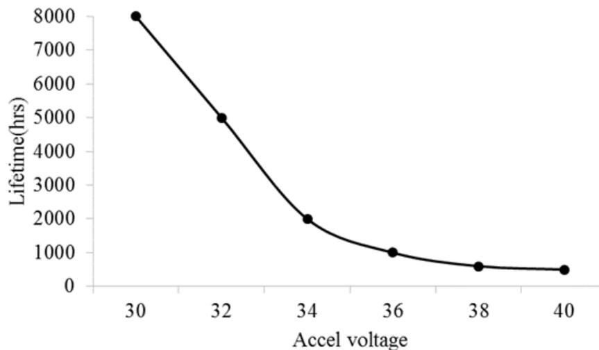
**Figure 3:** Impact of accelerator grid voltage on lifetime of ion thruster
