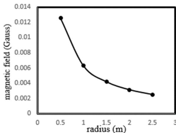
**Figure 5:** Variation of magnetic field with aperture radius of accel grid
