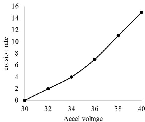
**Figure 2:** Impact of accelerator grid voltage on the erosion rate of ion thruster
