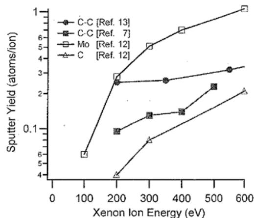
Figure 4: Comparison of Sputter Yields for Thrust Grid Materials
