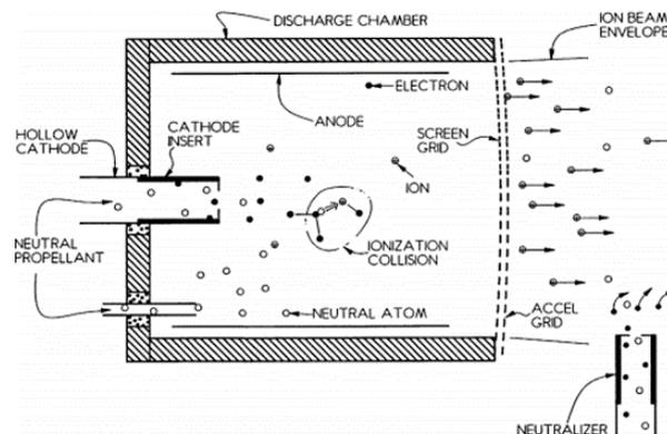
**Figure 1:** Schematic of ion thruster
