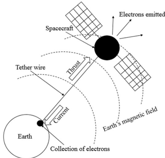
**Figure 6:** Representation of Electrodynamic Tether system to power spacecraft
