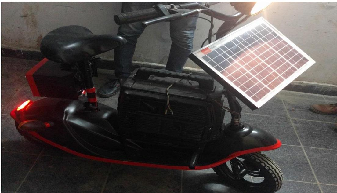
Fig. No 2.4(g) Final assembly of Two-Wheeler Series Hybrid Vehicle
