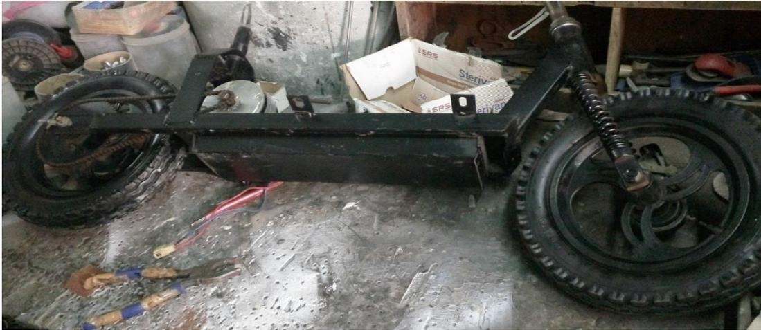
Fig No. 2.3(f) Assembling of front wheels into the frame along with shock absorber
