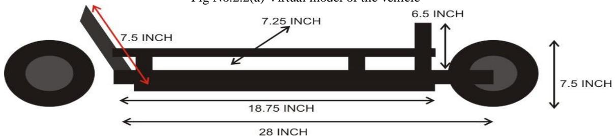
Fig no:- 2.2(b) Frame of the vehicle
