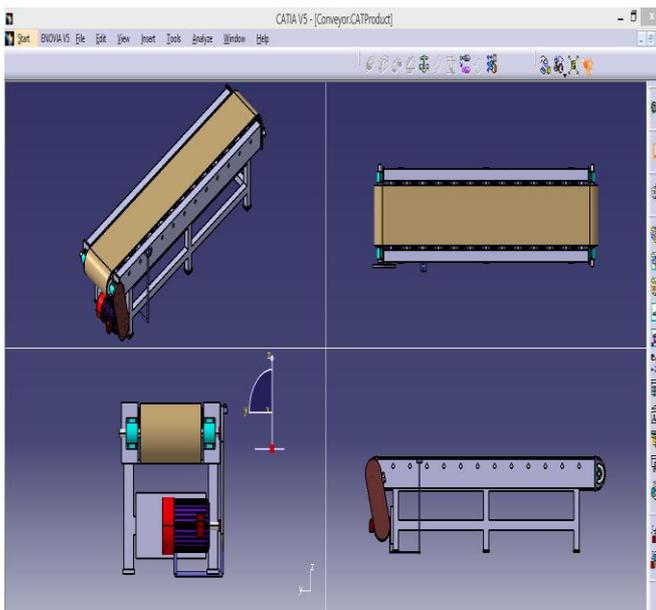
Fig.2. Conveyor Model in CATIA V5
