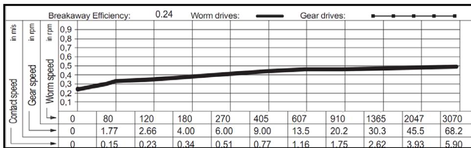
The most important factor in worm gear energy losses are losses from friction which differ from each other when the driving element is the worm and the worm wheel. The efficiency is strictly dependent on the lead angle and the friction coefficient between the worm and the worm wheel. Moreover in some special cases, the worm gear can become self-locking mechanism, this phenomena takes place when the lead angle is smaller than the apparent friction angle.
