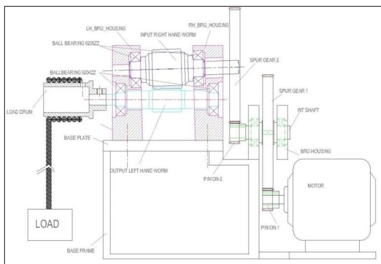
Fig: Worm pair system used in load lifting device
