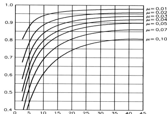
Fig: Efficiency vs Lead angle.
