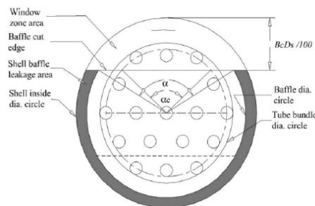
Figure 4: Illustration of baffle cut angles, leakage area.
