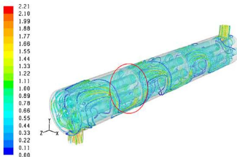
Figure 8: Velocity (m/s) path lines for 6 baffles (1 kg/s mass flow rate)
