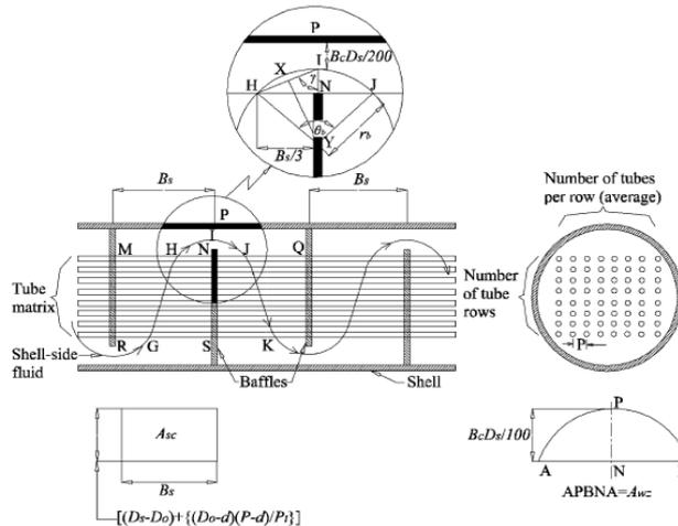
Figure 3: Showing the actual flow pattern in shell-side
