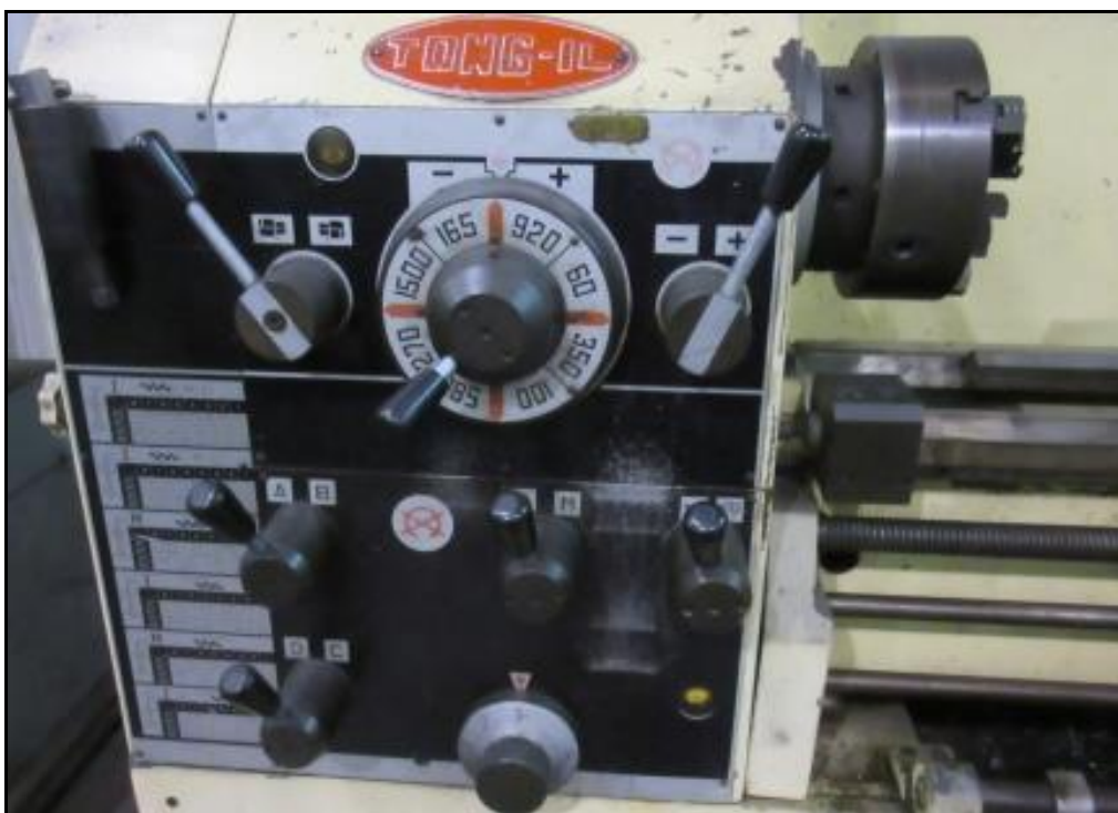
Fig. 1 TIPL-4 Lathe machine (Gear Arrangement)
