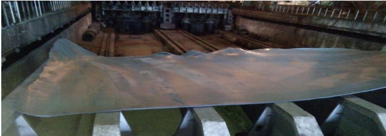
Fig 1 Edge Wave Defect in Steel Plate
