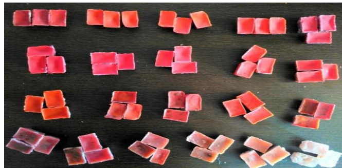
Fig 5 All Set of Cast Product Made from Mixing of Wax & Hot Melt Adhesive in weight%
