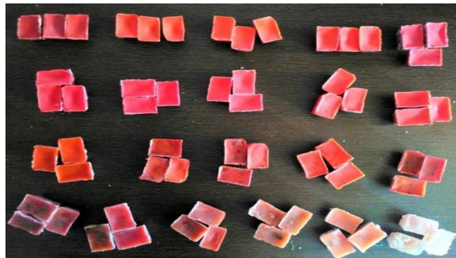
Fig 5 All Set of Cast Product Made from Mixing of Wax & Hot Melt Adhesive in weight%
