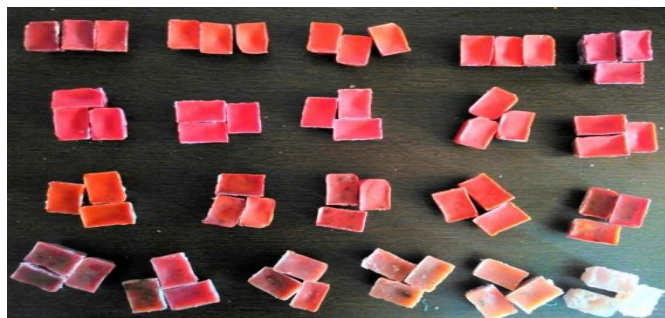
Fig 5 All Set of Cast Product Made from Mixing of Wax & Hot Melt Adhesive in weight%
