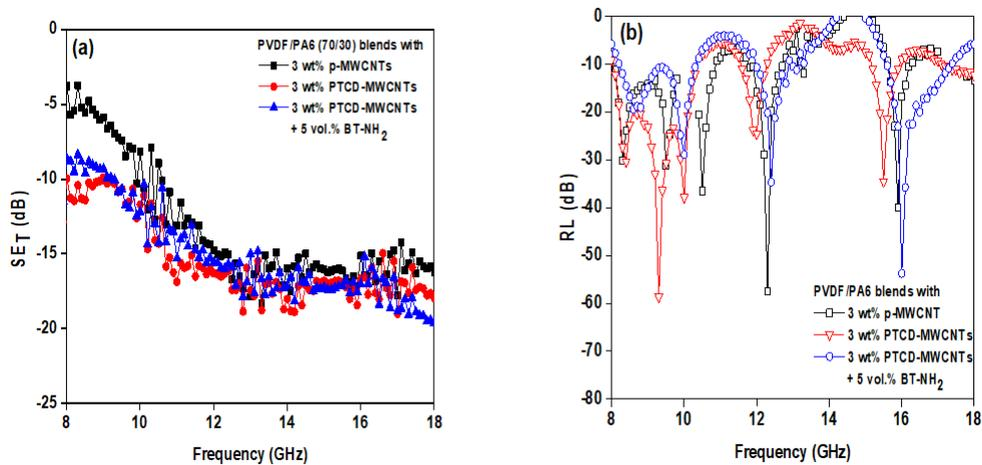
Figure 4: (a) Total shielding effectiveness as a function of frequency, (b) Reflection Loss as a function of frequency
