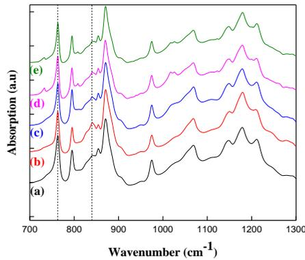
Figure 1: FT-IR Plot of (a) Neat PVDF, (b) Neat 70-30 PVDF-PA6 blends, (c) Blend with 3 wt. % p-MWCNT, (d) Blend with 3 wt. % PTC-D-MWCNT, (e) Blend with 3 wt. % PTC-D-MWCNTs+NH<sub>2</sub> functionalized BT
