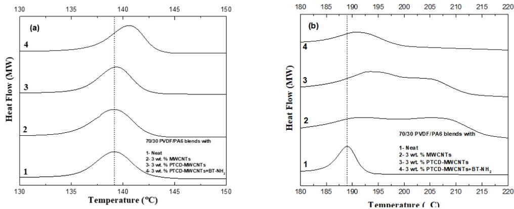
Figure: 2 DSC of (a) PVDF crystallization peak and (b) PA-6 Crystallization peak of different blend compositions
