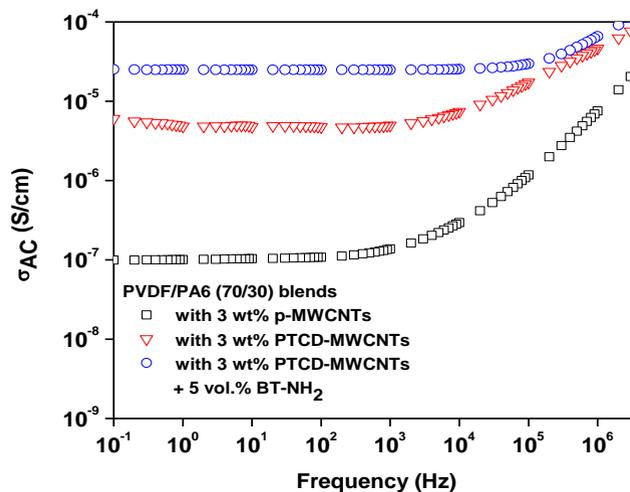
Figure 3: Room temperature AC conductivity as a function of frequency
