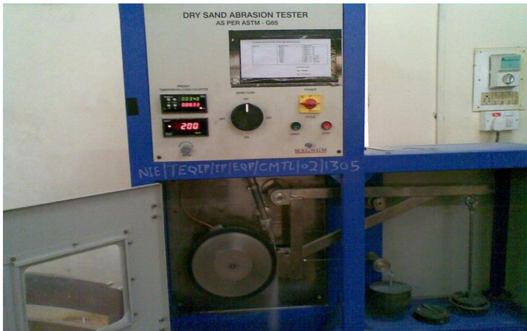
Fig 3.1. Three body abrasion tester
