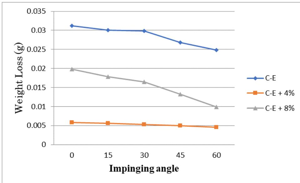
Fig 3.2: Weight loss Vs Impinging angle for C-E composites – With ageing
