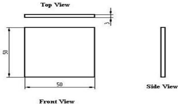
Fig 2.1. Air Jet Erosion Test Specimen
