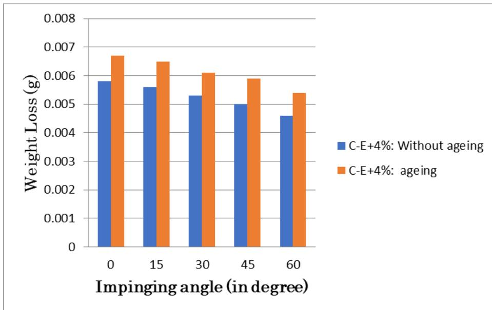
Fig 3.3: Comparison between aged and unaged C-E+4% filler composites: Air jet erosion test
