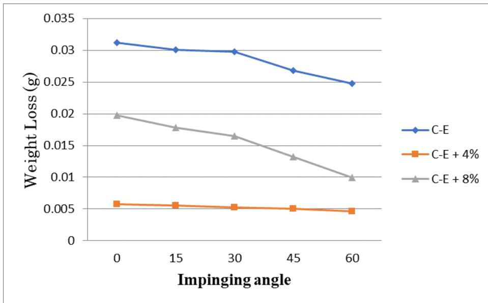
Fig 3.1: Weight loss Vs Impinging angle for C-E composites – Without ageing
