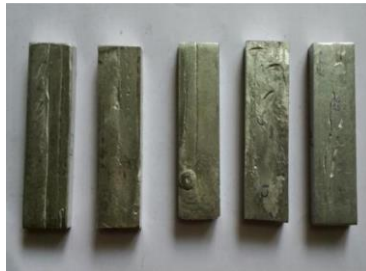
Figure 5: Specimen before Hardness Test
