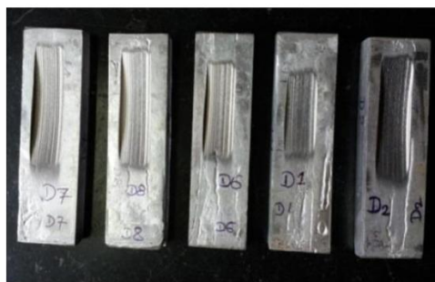
Figure 9: Specimen After Wear Test
