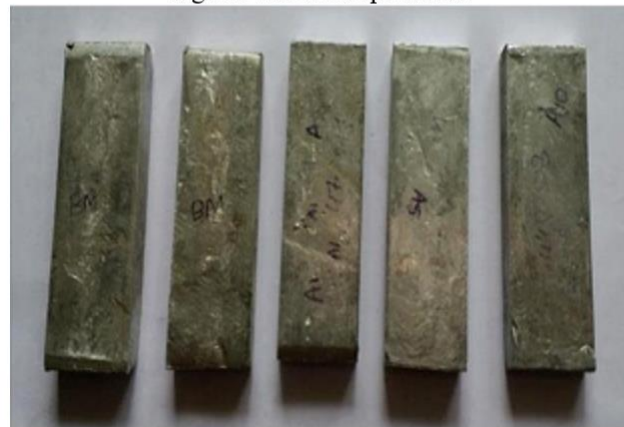
Figure 3: Specimen cut ASTM G-65 standards
