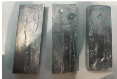
Figure 6: Specimen after Hardness Test
