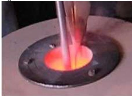
Fig 3.1: Stir casting Method
