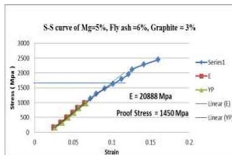
Fig 4.1.5: S-S Curve of composite for 3% fly ash, 6% graphite
