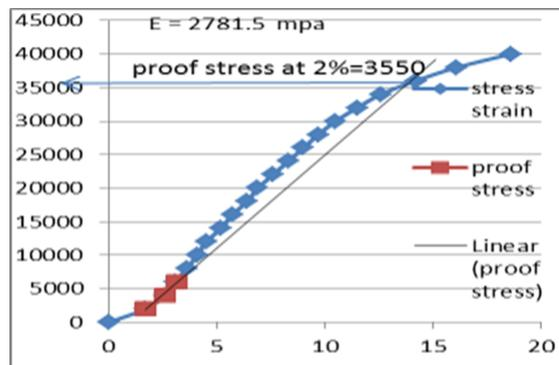
Fig 4.1.1: S-S Curve of composite for Al6061
