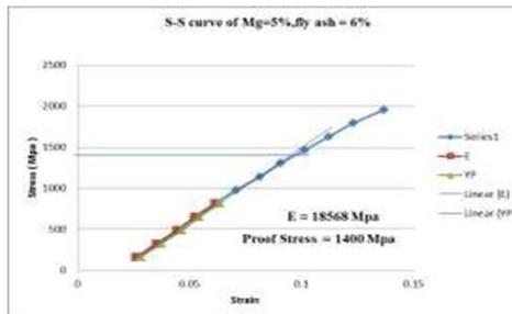
Fig 4.1.3: S-S Curve of composite for 6% fly ash
