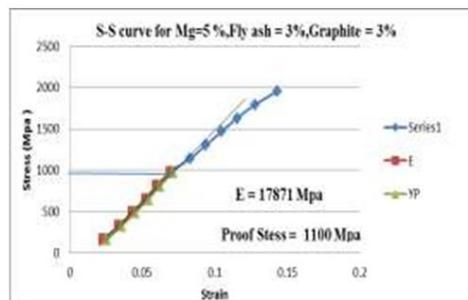
Fig 4.1.4: S-S Curve of composite for 3% fly ash, 3% graphite
