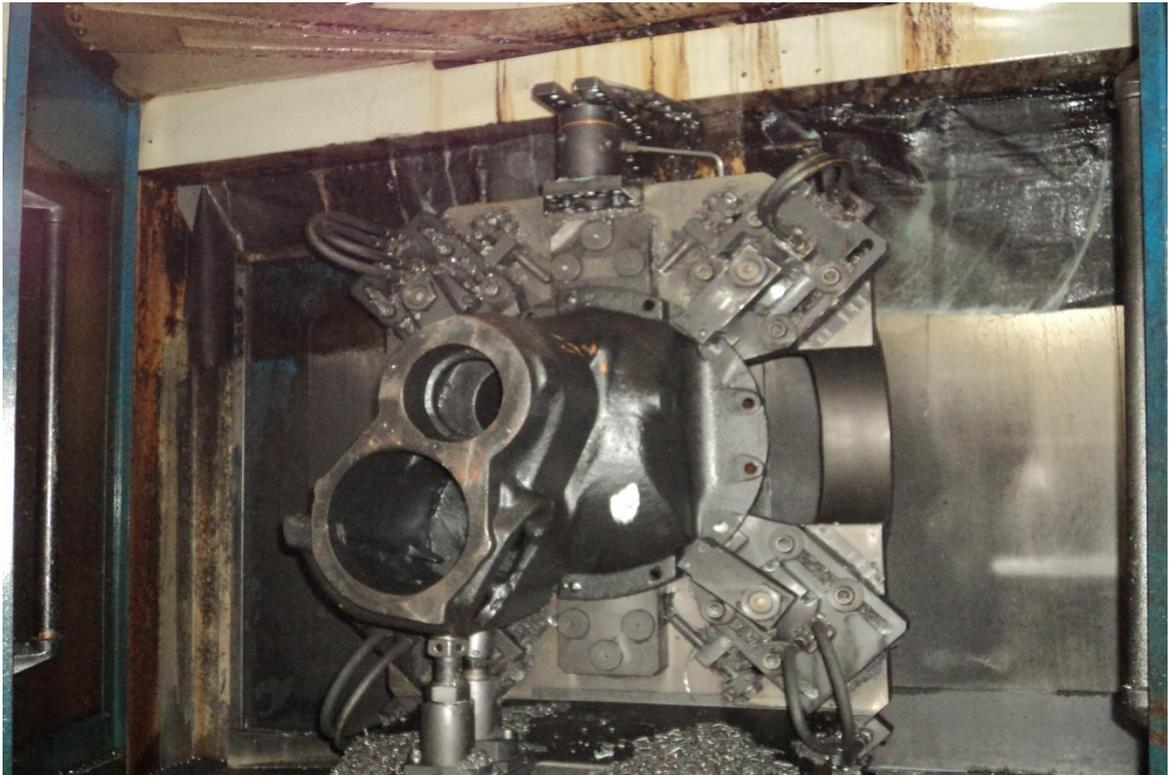
Fig 9.1: Job Mounting through Hydraulic Clamping
