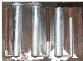
Figure 2: Final prepared composites in iron mould
