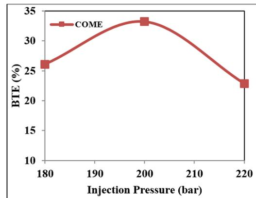
Fig 3: Variation of BTE Vs Injection Pressure
