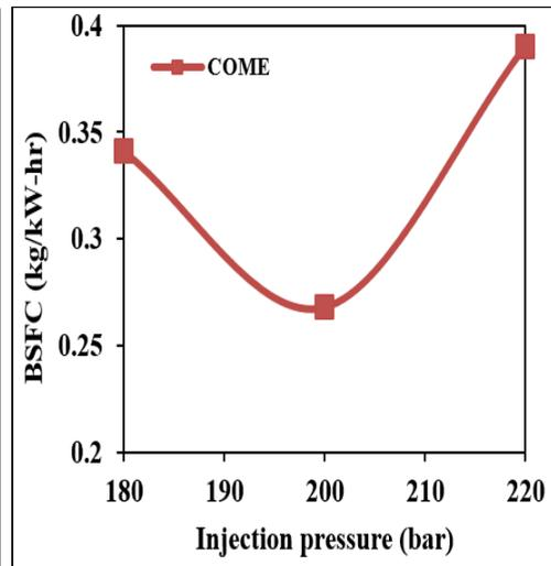
Fig 5: Variation of BSFC Vs Injection Pressure
