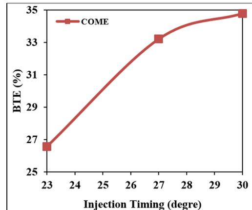
Fig 7: Variation of BTE Vs Injection Timing
