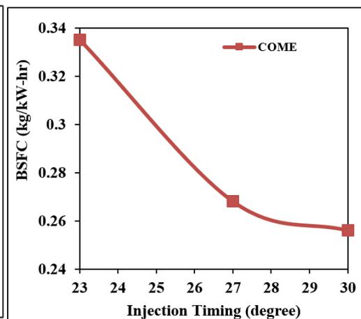
Fig 9: Variation of BSFC Vs Injection Timing
