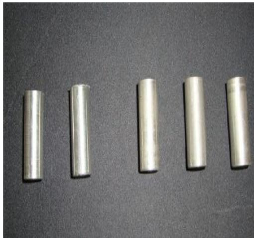
Figure 2: Wear Testing Specimens
