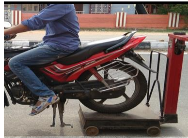
Fig.3. weighing rear tyre contact forces by lifting
