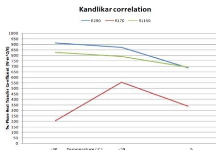
Fig.1: shows the variation of 2phase HTC with temperature for R290, R170, R1150 using Kandlikar correlation.
