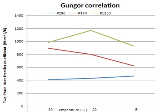
Fig.3: shows the variation of 2phase HTC with temperature for R290, R170, R1150 using Gungor correlation
