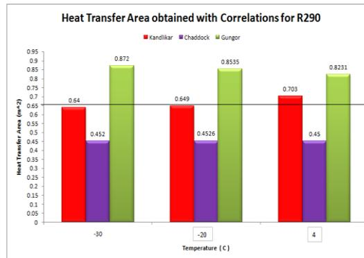
Fig.4: shows the Heat Transfer areas obtained from Kandlikar, Chaddock and Gungor correlation at working temperatures for R290.
