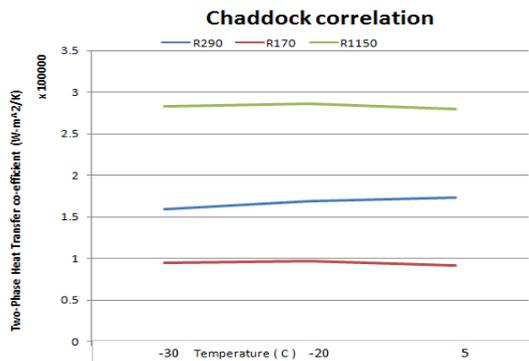
Fig.2: shows the variation of 2phase HTC with temperature for R290, R170 and R1150 using Chaddock correlation.
