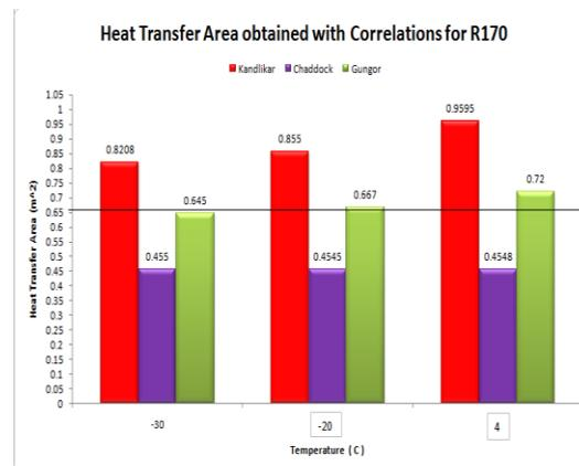
Fig.5: shows the Heat Transfer areas obtained from Kandlikar, Chaddock and Gungor correlation at working temperatures for R170
