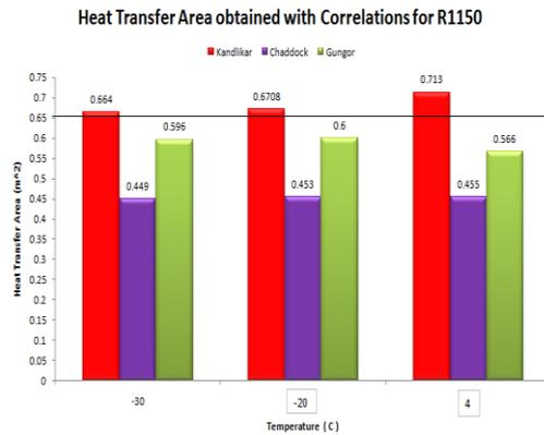
Fig.6: shows the Heat Transfer areas obtained from Kandlikar, Chaddock and Gungor correlation at working temperatures for R1150.
